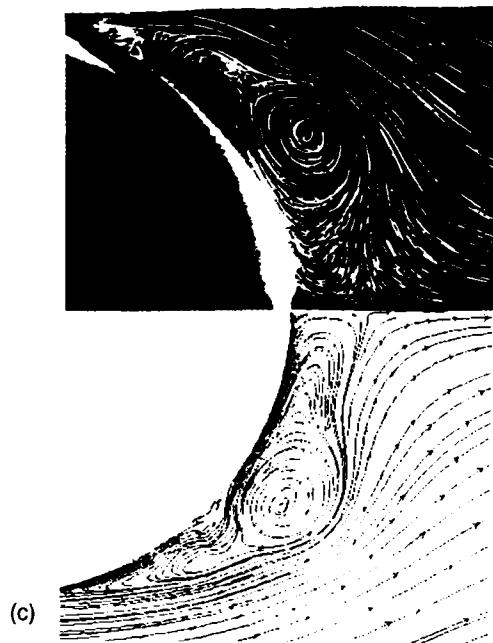
Figure 11(c). Impulsive start of circular cylinder at Re = 9500 . Comparison of particle traces 1,3 (upper part) with computed streamlines (lower part) at t = 1.25
